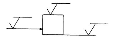
3.5 The maximum roughness number shall be placed adjacent to and on the inside of the long leg, as shown. Ref. Paragraph 2.10
