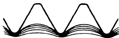
FLOW LINES, ROLLED THREAD FIGURE 3
