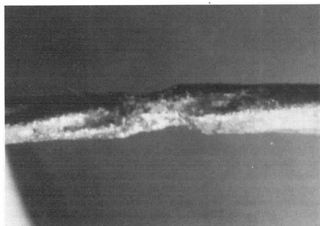
Figure 14-6.2(c) Stranded copper conductor in which melting by fire caused the strands to be fused together.
