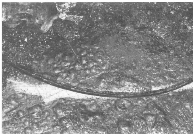
Figure 8-2.5.6(b) Floor tile protected from radiant heat by wire.
