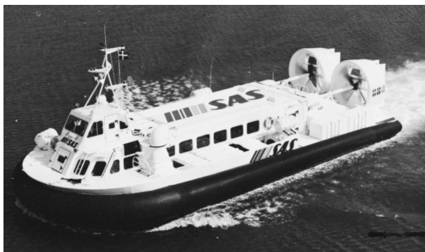
Figure A-3-16 The “Winchester” Class Hovercraft (built by the British Hovercraft Corporation), which is in service at the Auckland International Airport in New Zealand. It is utilized to protect aircraft operations that are largely over the Manukau Harbor that borders the airport. The primary mission is rescue of occupants in the event of an accident in the harbor or mudflats (which exist at low tide).
