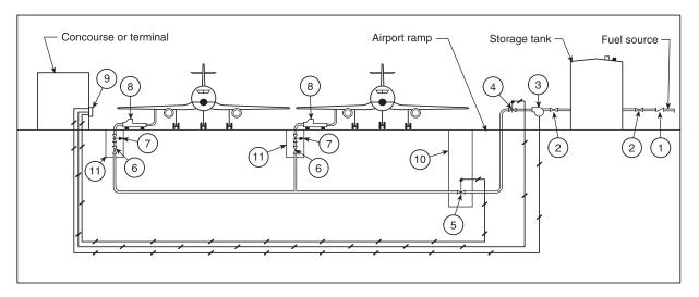
Note: No dimensional relationship exists between elements in this figure. Refer to this standard, NFPA 30, NFPA 70, and FAA Regulations for separations and clearances.
