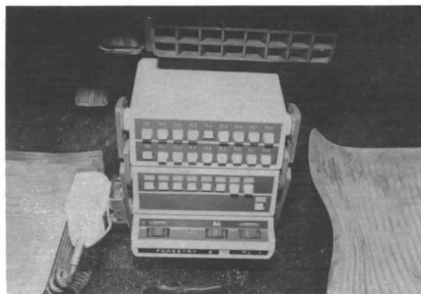
Solid state transmitter-receiver capable of 12-channel operation. Includes an 8-frequency scanner with 16-tone transmit capacity.
