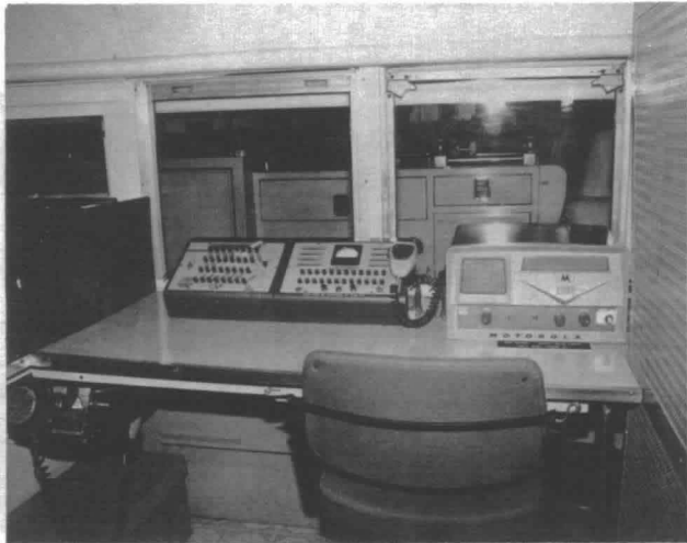
Radio operator's desk with cooperating agency's radio, tone encoder, and portable base station as installed in Mobile Incident Command/Communications Unit.
