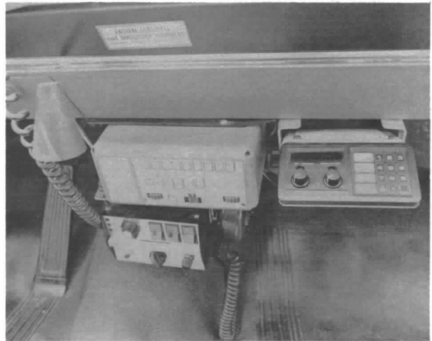
Left: four-frequency mobile radio control head with electronic siren/public address system below. Right: 20-frequency programmable scanner as mounted in sedan.
