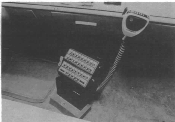
32-channel synthesized mobile transmitter-receiver unit. Mobile unit also includes an 8-channel scanner with two levels of priority and is capable of 16 tones on any of the 32 transmit frequencies.
