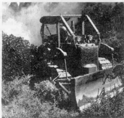
Tractor, angle dozer equipped and cable operated. Angle dozers may be positioned to operate as straight dozers. Brush guards are recommended for tractors which are to be used in the woods. All tractors shall be equipped with effective spark arrestors and protective canopies.
