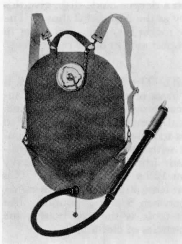
Bag-type back-pack pump. Capacity, 5 U.S. gallons; weight, 5 pounds.
