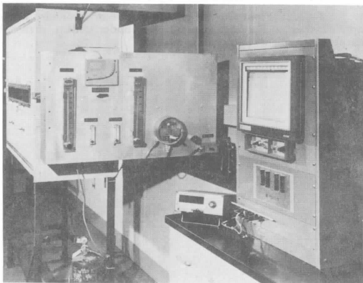
Figure 2-1A Flooring Radiant Panel Tester Apparatus.
