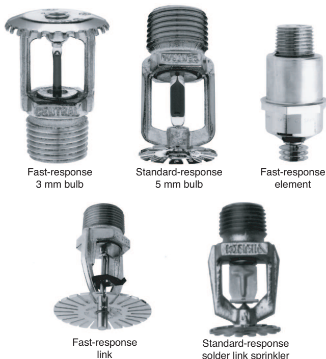
FIGURE A.5.3.1.1 Sprinkler Operating Element Identification.
