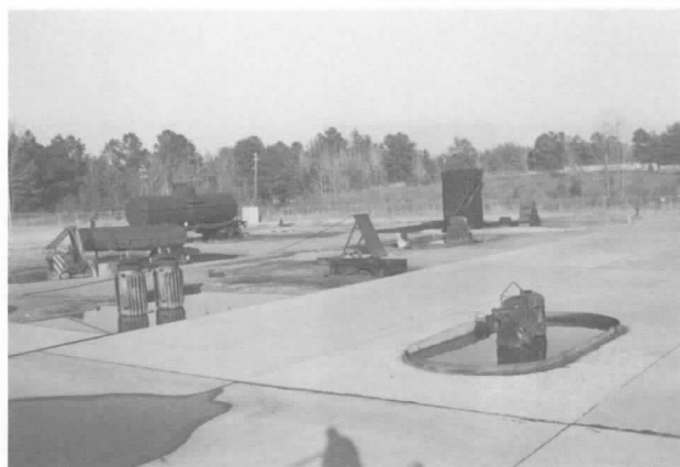
Figure 11-2 Flammable liquid burn area. Area includes cross pit, oval pit, square pit, electrical transformers, baffled pit, running spill area, drum pit, vertical tank, horizontal tank and railroad tank car. Mississippi Fire Academy.
