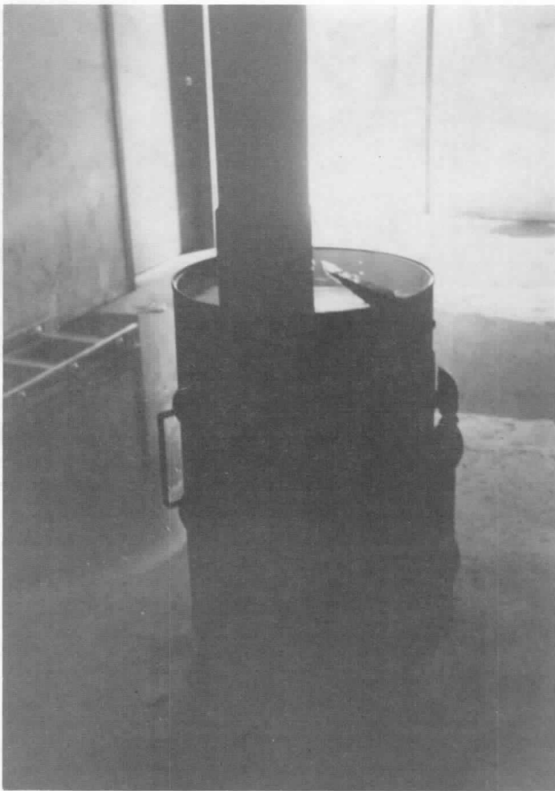
Figure 9-4.1 Smokemaking machine — very simple 55-gal (209-L) drum with hinged door half and smoke pipe to rooms on various floors.
