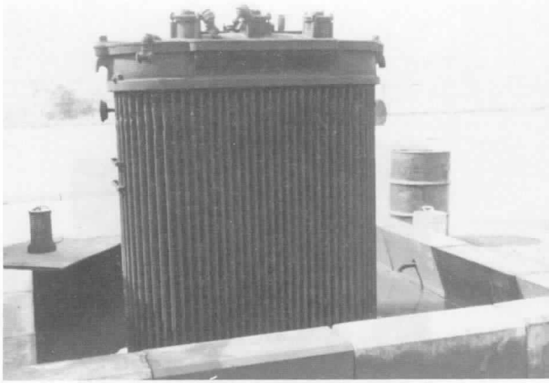
Figure 11-2.3(e) Flammable liquid cooled electric transformer mock-up. Note diking to contain runoff.
