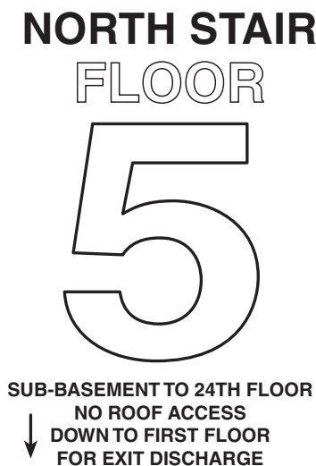
FIGURE A.10.11.3 Example of a Stairway Marking Sign. [101: Figure A.7.2.2.5.4]
