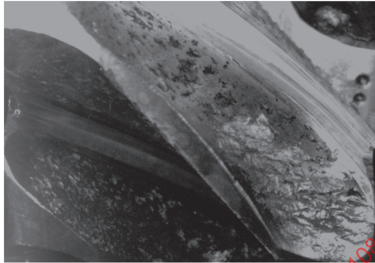
Figure 7 — Macropitting in progress for a very high lead angle worm gear set
