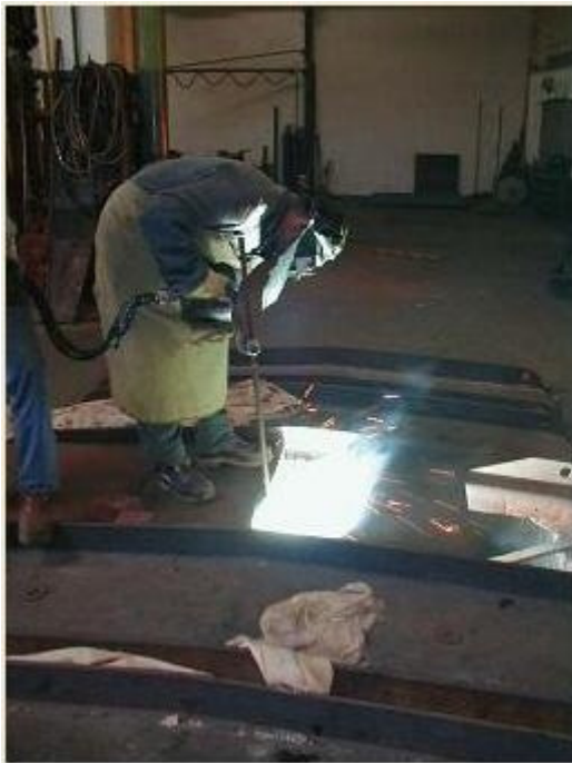
Figure 32 — A casting electrode is used to liquefy the peripheral zone of the parent metal
