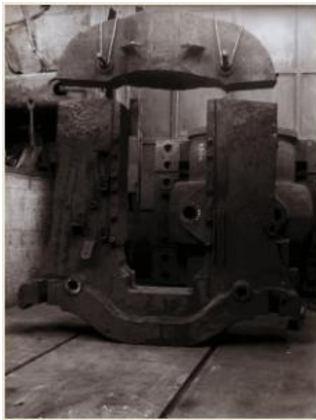
Figure 37 — Screw press column before repair welding
