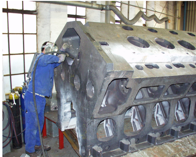
Figure 11 — Finishing welding at the 18-cylinder engine block
