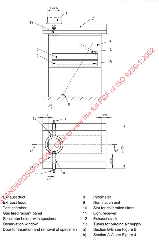
Figure C.2 — Side (B-B) and plan view of test equipment
