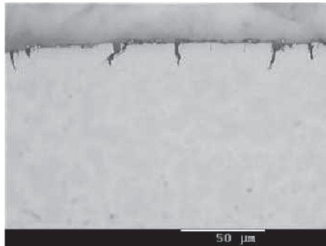
Figure 4 — Optical micrographs showing Ti3Al2.5V tube surfaces of deformed sections micro-cracks initiated in a diffusion zone
