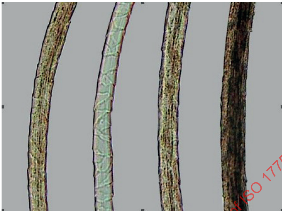
Figure C.35 — Irregular scales with thicker scale edges
