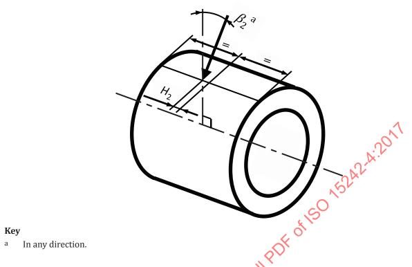
$Figure \, 1 - Radial \, load \, direction \, deviation \, in \, relation \, to \, direction \, and \, axial \, position$
