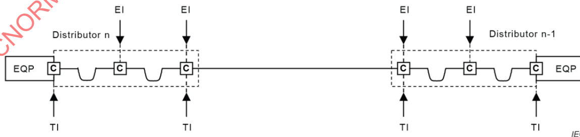
Cabling subsystems 2, 3 and 4
