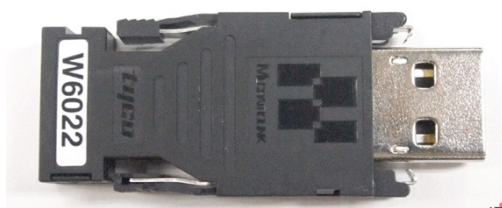
Figure A.10 – Terminator installed in M-II cable connector
